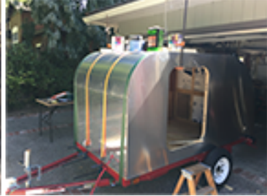
Skinned the roof
