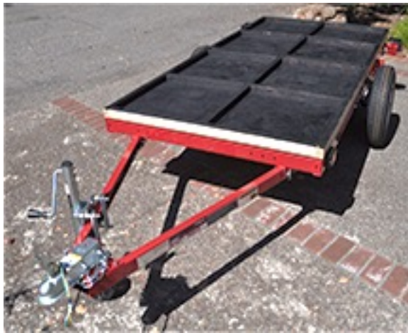
Upside down floor with road tar sealant
