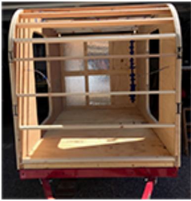
Spars attach the two sides
