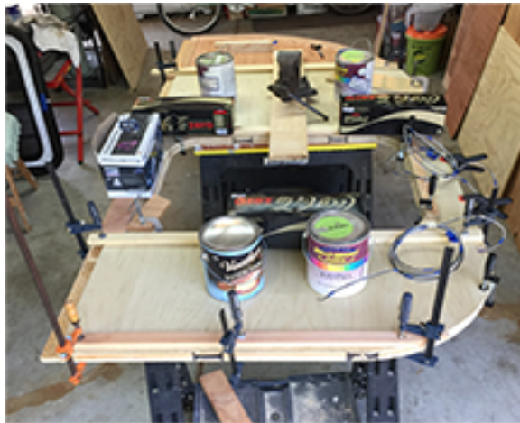
Gluing down the Luan interior wall
