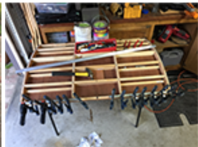
Gluing the inside Luan
